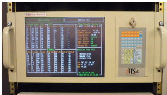
GNSS-receiver: reception of GPS, GLONASS and GALILEO
