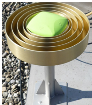
Antenna (choke ring type) for the GNSS-receiver, mounted on the roof of our building
