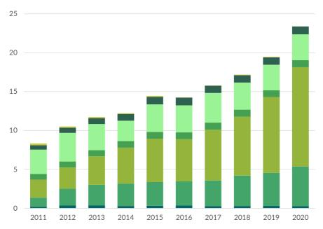
The production of renewable electricity grew strongly in the last decade. The production of electricity based on solar energy shows a strong increase (+20.1%) for the third year in a row after a few years of stagnation. Production on the basis of solid biofuels has recovered since its decrease in 2014 and reached a high in 2017 at 3.8 TWh. Between 2019 and 2020, wind production increased by 30.9%.
