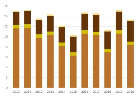
The primary energy production of renewables and biofuels has greatly increased from 2.5 Mtoe in 2011 (share of 16.7%) to 4.0 Mtoe in 2020 (share of 29.9%). This increase is mainly caused by new wind farms and solar panels. Between 2019 and 2020, wind production increased by 30.9% and solar production increased by 20.1%. Nuclear energy production decreased by 21.0% compared to 2019 due to a combination of technical problems and planned maintenance in the nuclear installations.
