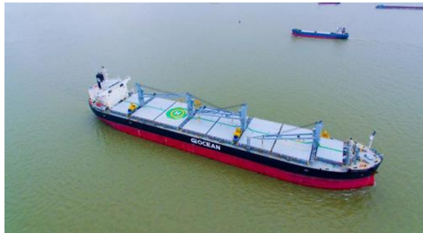
Figure 2-8 Open hatch bulk carrier (Project Cargo Weekly, 2018)
